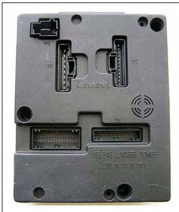
locate and read MC68HC05B16/32 Megane Immoibox Siemens (attached to the back of the fuse box):
