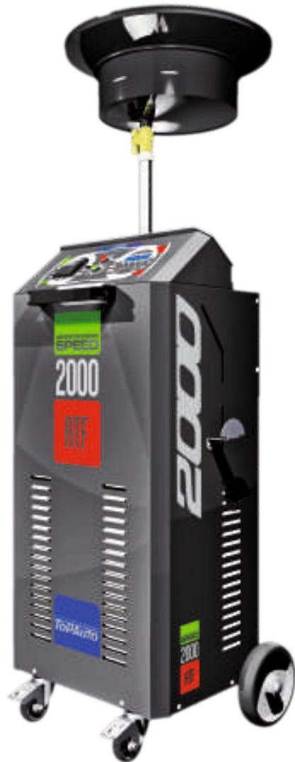
Safety management for proper oil level in the automatic transmission during oil changes. 12 Volt variable flow pump that adapts automatically to the flow speed of any type of gearbox, avoiding the possibility of having a different speed between the car pump and the ATF pump; weighing of new and exhausted oil through the scales underneath the tanks; all this means you have nothing to do, nothing to be worry. The machines makes correctly and carefully the replacement of the oil.
